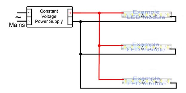
Advantages of this solution is very low voltage of power supply and uniform distribution of light. It meets requirements of SELV. Higher current supply is required to proper operation. Higher current increases temperature and decreases lifetime. Above connection is example and may be different from the actual.
