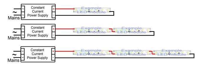
Advantages of this solution are very effective operation and uniform distribution of light. Higher voltage supply is require, when large number of LED modules are connected. If too many LED modules are connected, the voltage value may not meet requirements of SELV. Non-SELV voltage need additional protection. All above connections are examples and may be different from the actual.
