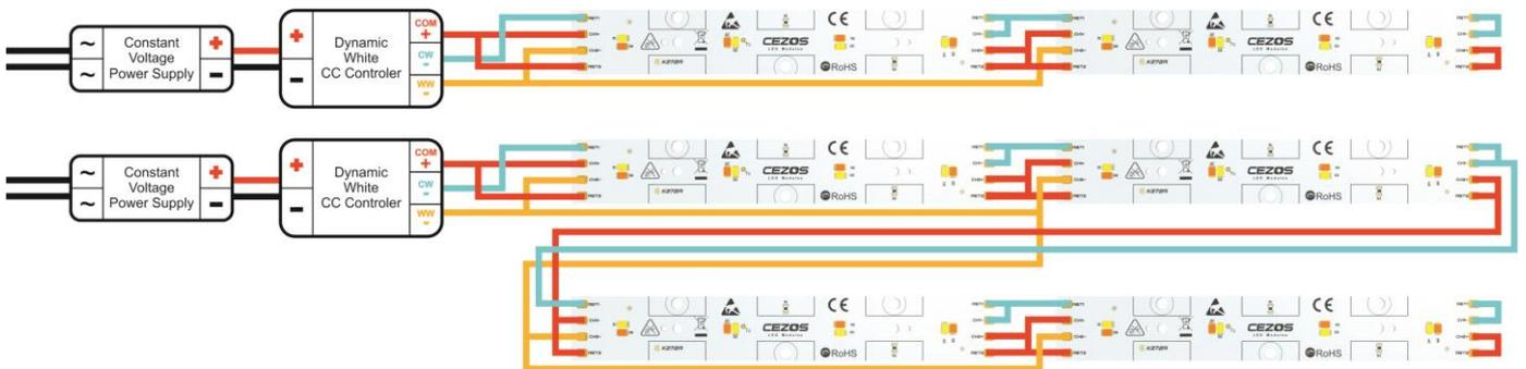
To meet SELV requirements LED modules may be connected with serial-parallel wiring, maximal two LED modules in serial. Advantages of this solution are lower voltage and higher current.
