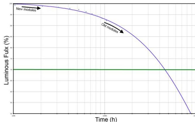
Most common problem using new modules in old installation is differences in brightness of modules. This is result of luminous flux degradation over time of use. Degradation is normal effect and applies to all LEDs. This effect is different for each LEDs and can be only predicted by testing and estimation. It is complicate issue that mostly depends on temperature and current. Good solution to this problem is reduce of current in new modules, but
