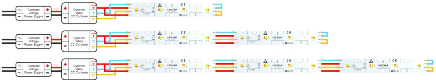
Advantages of this solution are very effective operation and uniform distribution of light. Higher voltage supply is require, when large number of LED modules are connected. If too many LED modules are connected, the voltage value may not meet requirements of SELV. Non-SELV voltage need additional protection. All above connections are examples and may be different from the actual.
