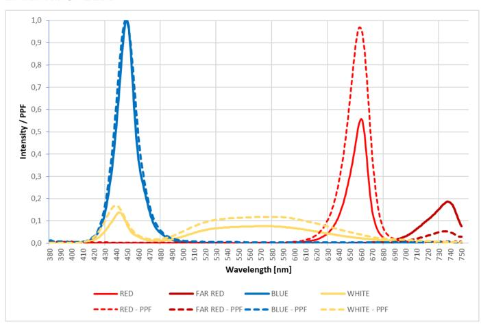
Normalized spectrum graph of the red, far red, blue and white LEDs at 700 mA current. Spectrum can be changed by choosing LEDs and power output.
