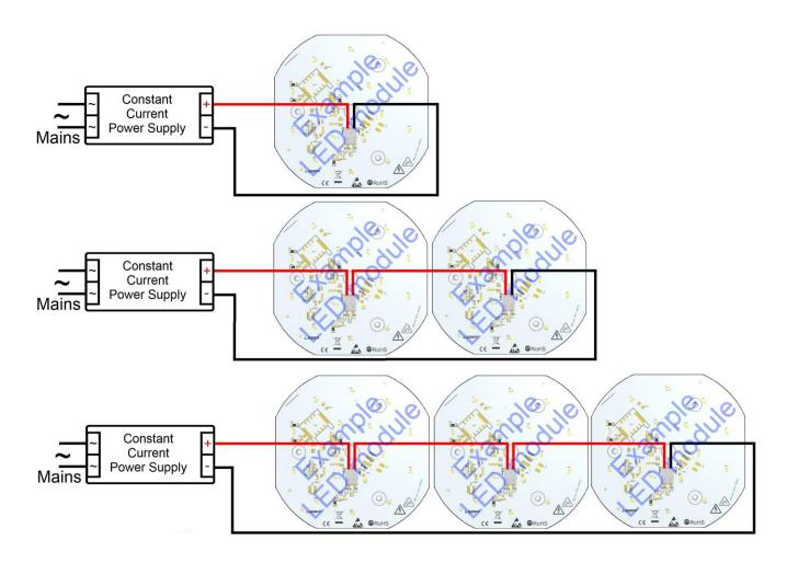
Advantages of this solution are very effective operation and uniform distribution of light. Higher voltage supply is require, when large number of LED modules are connected. If too many LED modules are connected, the voltage value may not meet requirements of SELV. Non-SELV voltage need additional protection. All above connections are examples and may be different from the actual.
