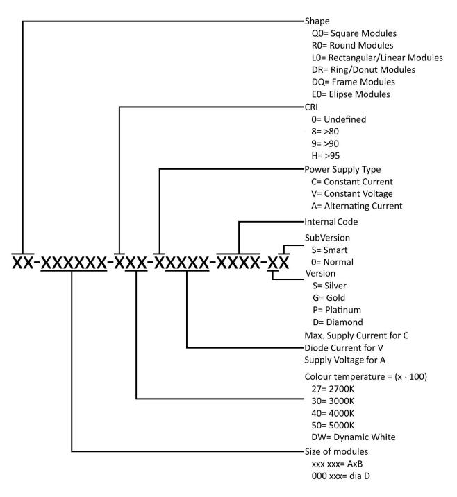
Above description of article number is standard for white modules, but it may be different. If modules doesn't have any version or subversion, than last two position are skipped. RGB/RGBW modules have in places of CRI written "R" and modules without white LEDs have "GB" in colour temperature. Additionally position of version is skipped.
