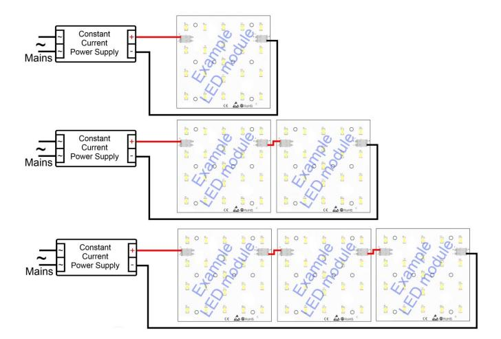
Advantages of this solution are very effective operation and uniform distribution of light. Higher voltage supply is require, when large number of LED modules are connected. If too many LED modules are connected, the voltage value may not meet requirements of SELV. Non-SELV voltage need additional protection. All above connections are examples and may be different from the actual.
