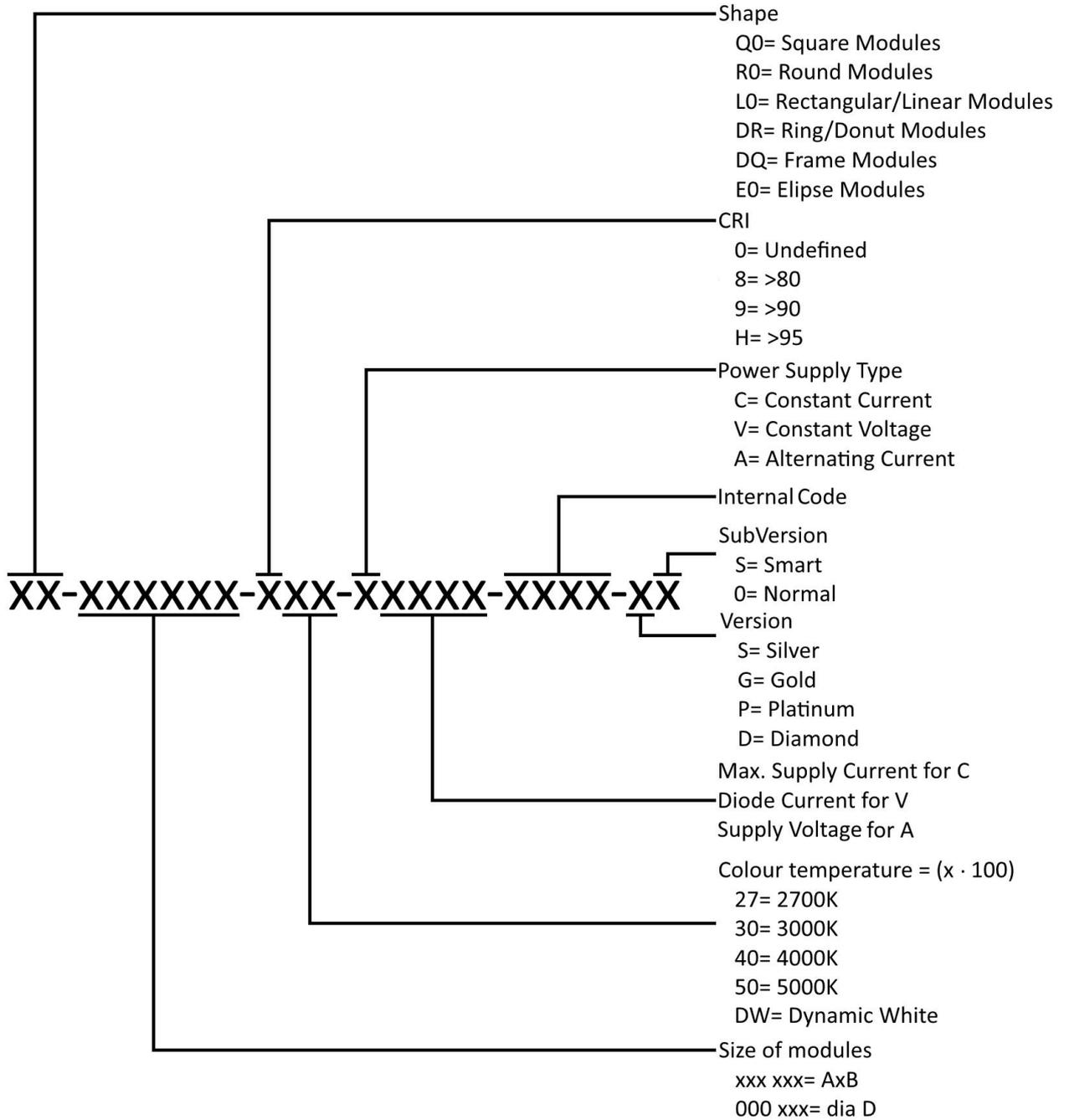
Above description of article number is standard for white modules, but it may be different. If modules doesn't have any version or subversion, than last two position are skipped. RGB/RGBW modules have in places of CRI written "R" and modules without white LEDs have "GB" in colour temperature. Additionally position of version is skipped.
