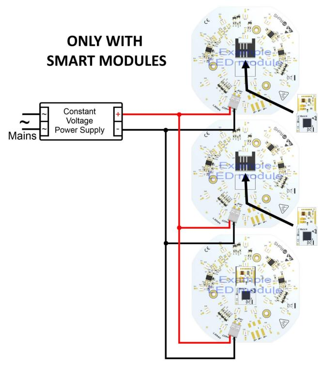
This is special wiring available only for SMART modules. Connecting external controller is not allowed and they don't work properly without compatible driver in the slot. Advantage of this solution is possibility to replace white LED modules without changing the existing installation.
