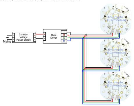
Advantages of this solution are very low voltage supply and uniform distribution of light. It meets requirements of SELV. Higher current supply is require to proper operation. Connections RGB LED modules with serial wiring is unacceptable. Such connection may damage or destroy modules. We are not responsible for any loss, or damage resulting from improper use of modules! Guarantee become void in such cases. Above connections are examples and may be different from the actual.
