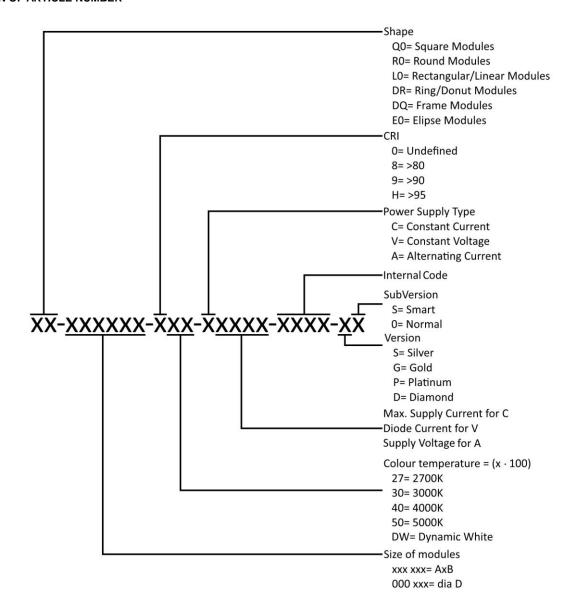
Above description of article number is standard for white modules, but it may be different. If modules doesn't have any version or subversion, than last two position are skipped. RGB/RGBW modules have in places of CRI written "R" and RGB have "GB" in colour temperature. Additionally position of version is skipped.
