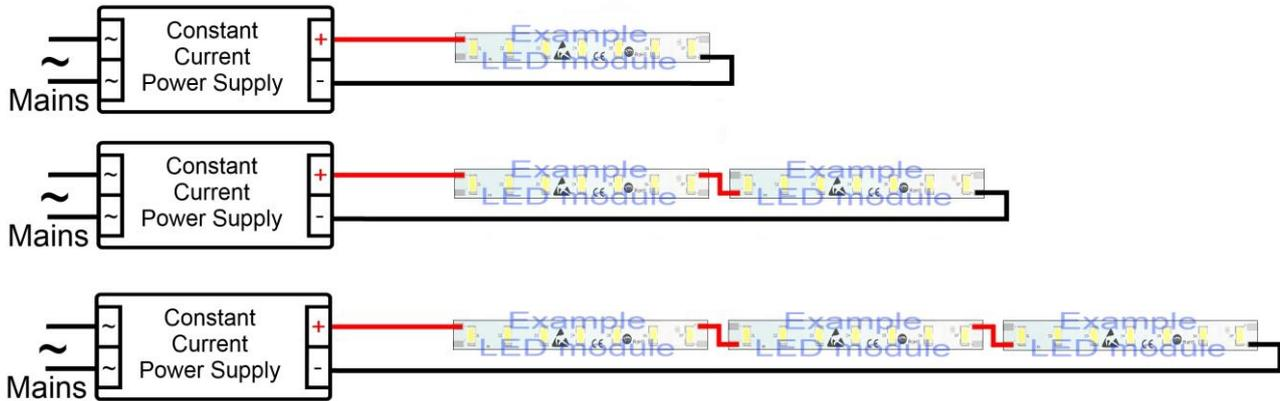
Advantages of this solution are very effective operation and uniform distribution of light. Higher voltage supply is required, when large number of LED modules are connected. If too many LED modules are connected, the voltage value may not meet requirements of SELV. Non-SELV voltage need additional protection. All above connections are examples and may be different from the actual.
