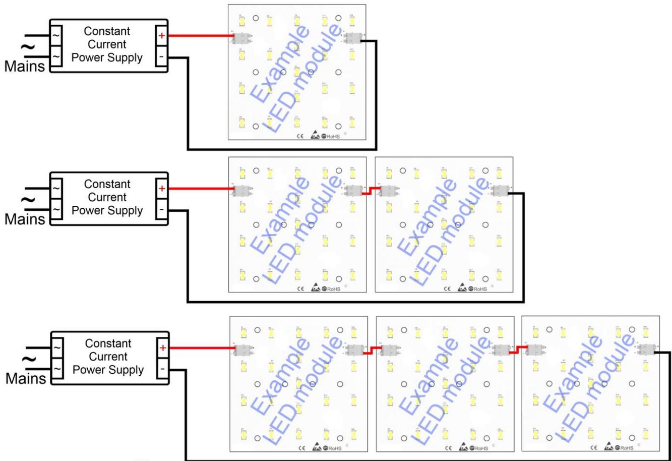
Advantages of this solution are very effective operation and uniform distribution of light. Higher voltage supply is required, when large number of LED modules are connected. If too many LED modules are connected, the voltage value may not meet requirements of SELV. Non-SELV voltage needs additional protection. All above connections are examples and may be different from the actual.
