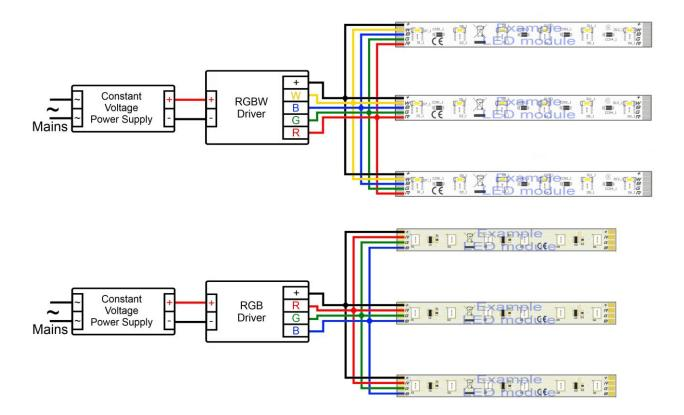
Advantages of this solution are very low voltage supply and uniform distribution of light. It meets requirements of SELV. Higher current supply is require to proper operation.
