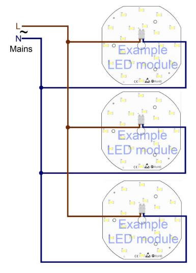
230V AC LED modules can be connected only in parallel. Series connection is unacceptable. We are not responsible for any loss, or damage resulting from improper connections! Guarantee become void in such cases. Above connection is examples and may be different from the actual.
