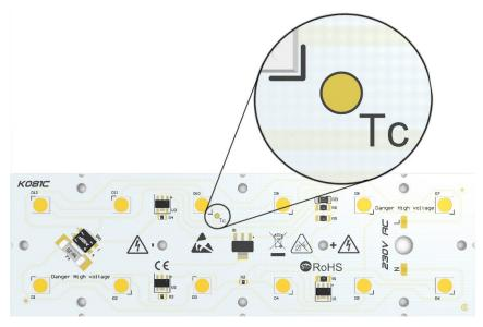
Temperature test point ( $T_c$ ) for measurement is usually localized in the middle of the board near LED's thermal pad. The temperature at the  $T_c$  point can be measured with thermocouple or simple temperature probe. Example of  $T_c$  point is shown on the photo above. If the module is potted, temperature should be measured on the edge of the board. If temperature at  $T_c$  will be lower than 65°C, the value of luminous flux shouldn't be less than 80% of its nominal value after 50.000h.
