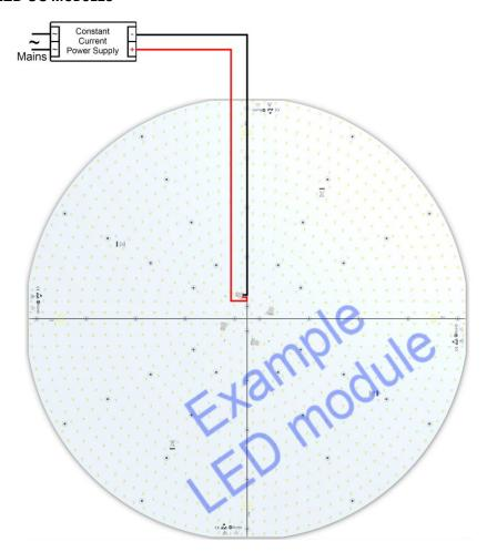
This LED modules should be connected to two power supply or drivers. It allow to independently control sets of LEDs. Same channels of couple LED modules may be connected with serial or serial-parallel wiring. Higher voltage supply is require, when large number of LED modules are connected. If too many LED modules are connected, the voltage value may not meet requirements of SELV. Non-SELV voltage need additional protection All above connections are examples and may be different from the actual.
